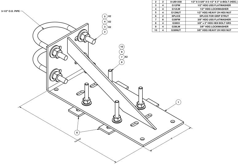
**TOLERANCE NOTES** TOLERANCES ON DIMENSIONS, UNLESS OTHERWISE NOTED ARE: SAWED, SHEARED AND GAS CUT EDGES (\$ 0.030") ORILLED AND GAS CUT HOLES (\$ 0.030") - NO CONING OF HOLES LASER CUT EDGES AND HOLES (\$ 0.010") - NO CONING OF HOLES BENDS ARE ± 1/2 DEGREE ALL OTHER MACHINING (± 0.030") ALL OTHER ASSEMBLY (± 0.060") PROPRIETARY NOTE:
